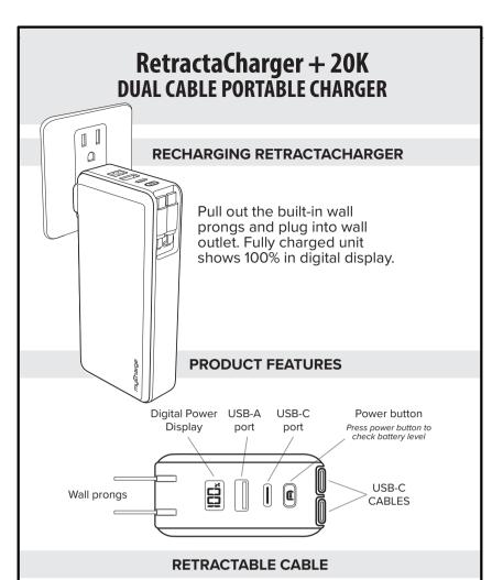
Pull out the built-in USB-C cable to desired length and plug into device. Charging should begin automatically – if
